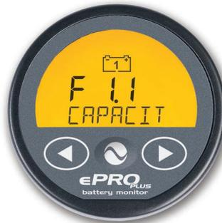
During function setup, status or history readout, each parameter is clearly explained using scrolling text in the display. This will make it a lot easier to browse through the ePRO Plus menu, without having to consult a list of parameter numbers.
