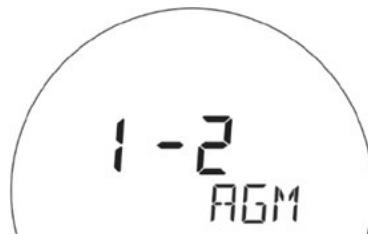
The display will start by showing the battery type selection screen. You can use the left (<) and right (>) arrow keys to select between AGM (default), GEL, Flooded and Lithium LiFePO4. Please consult your battery manual or supplier, to find out the correct type of your battery system. Once the selection has been made, press the MENU key to jump to the next step.
