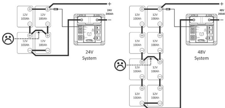
The reason for this is that through the interconnected midpoints, one bad battery in a series string can damage all other batteries if not being monitored correctly. However, when decent midpoint voltage measurement has been applied and an alarm is triggered when the voltage difference is too large, the midpoints of the series strings are allowed to be interconnected. This will result in the following connection diagrams:
