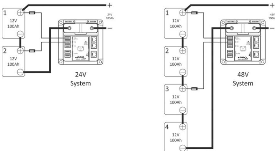
Please note that when using the +B2 input for midpoint voltage measurement, you should set Function F2.0 to 'MIDPNT'. You can also configure the +B3 input for midpoint voltage measurement, but only one of these two inputs can be used at the same time for this purpose.
