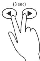
Besides automatic synchronisations, you can also manually synchronize the battery monitor, when you are sure that your battery is fully charged. This can be accomplished by pressing both left and right arrow keys simultaneously for three seconds. After these three seconds, the SoC value will be reset to 100%.
