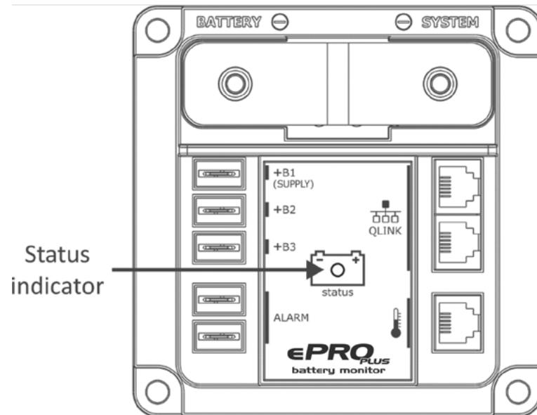
The status indicator has multiple operating modes, distinguished each by colour or flash interval. Please see the table below for an overview of the operating modes:
