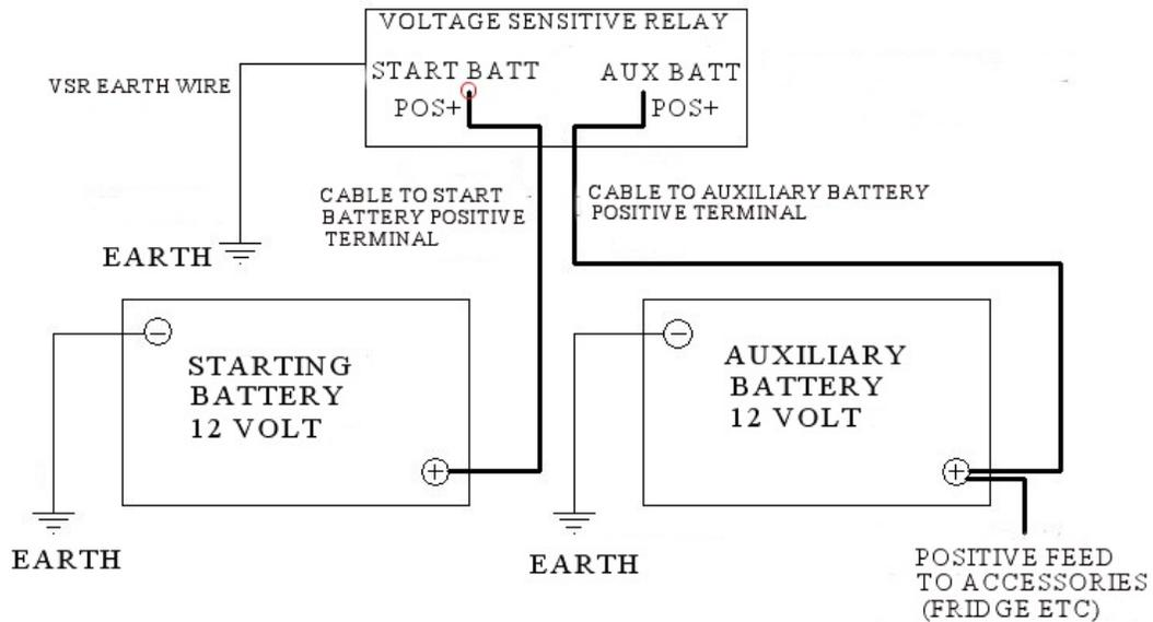
**6.** Take the 6 metre length of red cable, which has been terminated at both ends. Begin from the centre of the mounting plate and run the cable along the inner guard and firewall to the positive terminal of the starting battery (be careful to keep the wiring away from any moving parts). Cut the cable to length.
